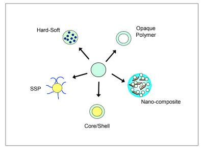
Figure 2. Acrylic polymer particle morphologies
